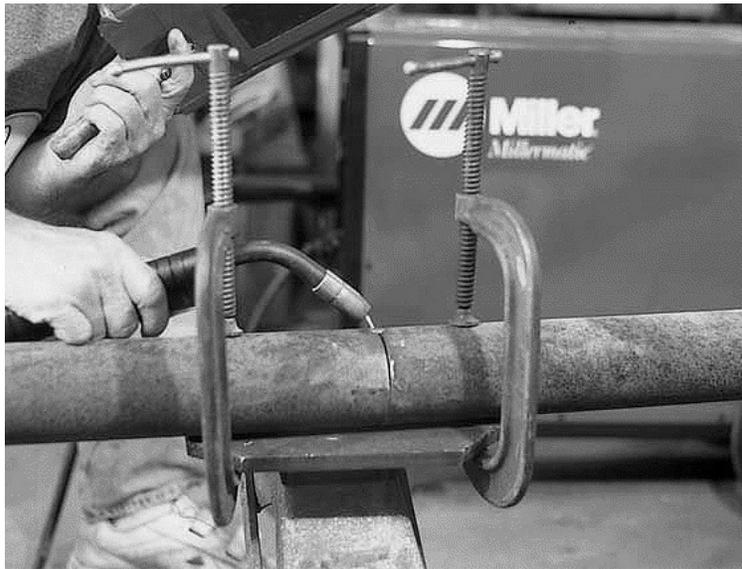
I used a piece of steel that wouldn't bend placed below the axle and two large "C" clamps.
